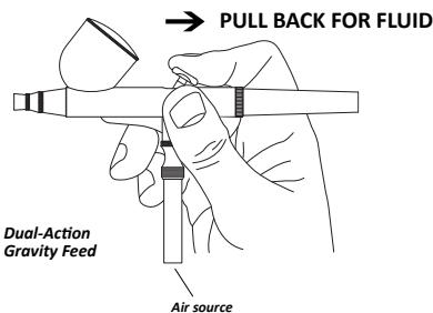
Dual-action airbrushes are the most widely used style of airbrush, as they allow the user to have superior control of the air flow, fluid flow and spray pattern. The three main dual-action airbrush types are Gravity Feed, Siphon Feed and Side Feed.
