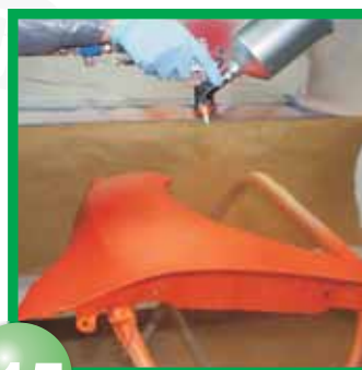
#15&16 Apply 2 to 3 medium wet coats of Auto Air Colors #4315. Allow coats to dry matte finish before re-coat, use waterborne dryer gun to assist dry time.
