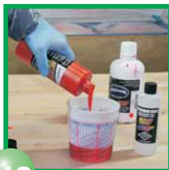
#12&13 Reduce 9:1 or 10% per volume with #4012 High Performance Reducer
