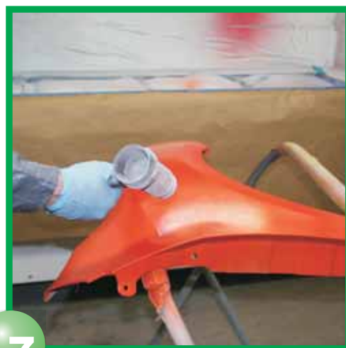
#12&13 Reduce 9:1 or 10% per volume with #4012 High Performance Reducer
