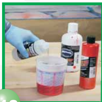
#12&13 Reduce 9:1 or 10% per volume with #4012 High Performance Reducer
