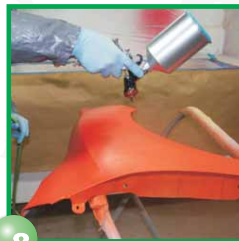
#14 Allow reduced paint to rest for approx. 10 minutes
