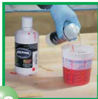
#2&3 Reduce 9:1 or 10% per volume with #4012 High Performance Reducer
