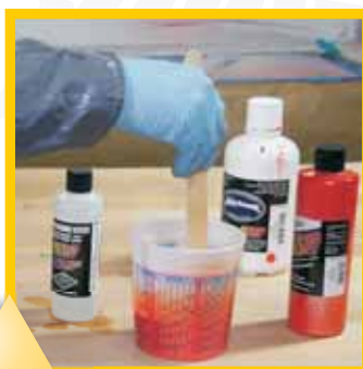
#14 Allow reduced paint to rest for approx. 10 minutes
