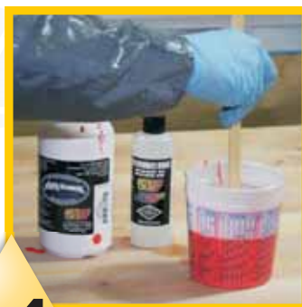
#4 Allow reduced paint to rest for approx. 10 minutes
