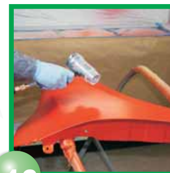
#15&16 Apply 2 to 3 medium wet coats of Auto Air Colors #4315. Allow coats to dry matte finish before re-coat, use waterborne dryer gun to assist dry time.
