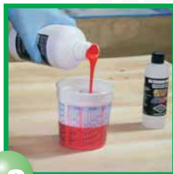
#2&3 Reduce 9:1 or 10% per volume with #4012 High Performance Reducer
